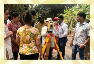
The resource person for the workshop was Mr. Anant Pawaskar from Allterra Solutions LLP, Vashi, Navi Mumbai. Mr. Anant covered basic training of centering and levelling of the total station on the very first day. He also explained Station setup resection /stake out operation station elevation, topo survey, counter survey, cogo function key in parameters, downloading and uploading job data exporting in different formats like CSV and DXF to pen drive. Dr. Shwetha Prasanna coordinated the workshop.
